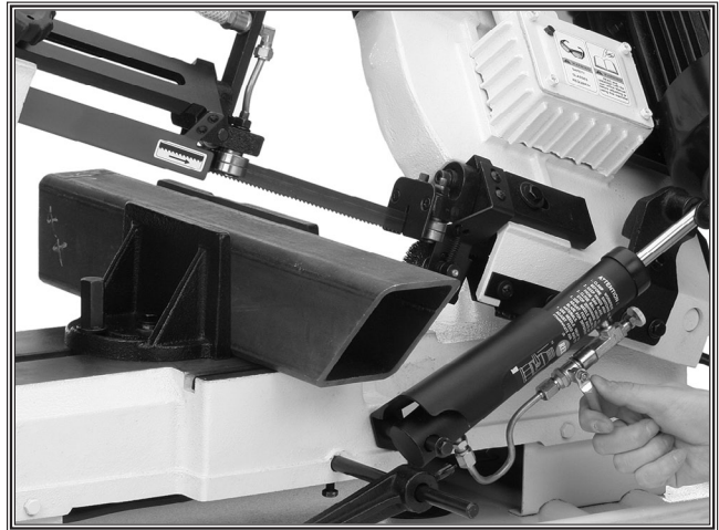
Figure 7. Always start the saw with the blade clear of the workpiece.
